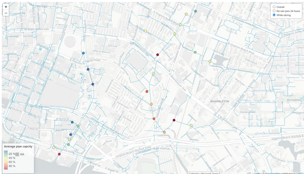
Figure 2. Two StormSensor® networks in Norfolk, VA, monitor flow on a continuous basis. Locations are color-coded according to how full the pipes are during a rain event. These sewersheds discharge into the Elizabeth River and are impacted by tides and sea level rise.
